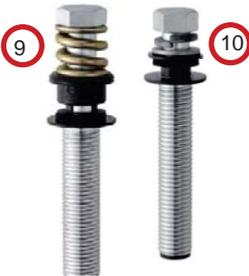
Hilti provides elastic fasteners if elastomeric pads are situated between rib plate and concrete surface. The necessary movement of the baseplate is ensured by Hilti DFF adapted with compression springs (9) which will be pre-tensioned during installation.
