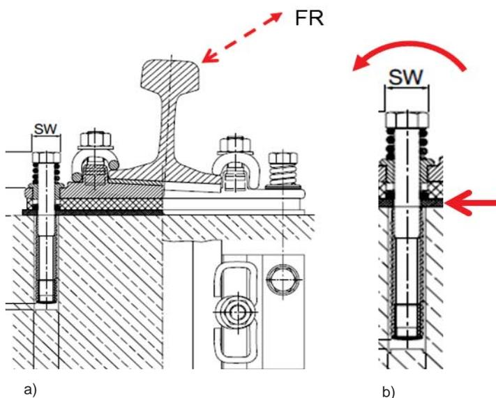
a) Cross section and inclined load  $F_R$  by rolling stock
