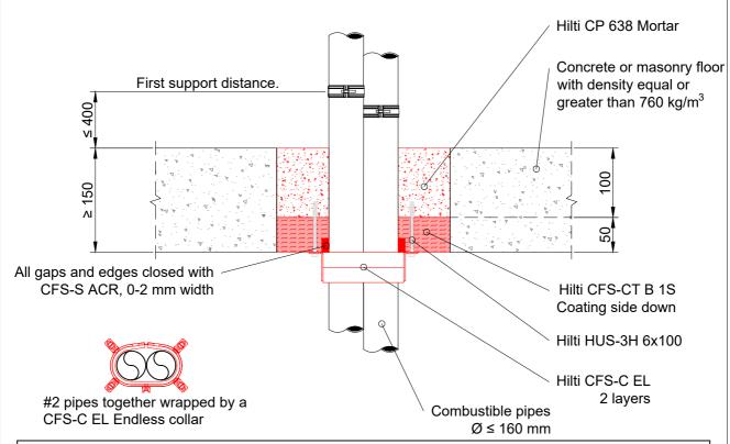
PE pipes in acc. EN 1519-1, EN 12201-1, EN 15494, EN 12666-1, PE-X pipes in acc. EN 15875-2, ABS pipes in acc. EN 1455-1 and EN 15493, as well as SAN+PVC in acc. ISO 19220.
