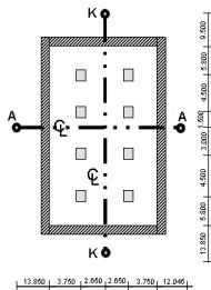
Height marks and control lines are generally marked out on and around the building plot by a surveyor before construction begins.
