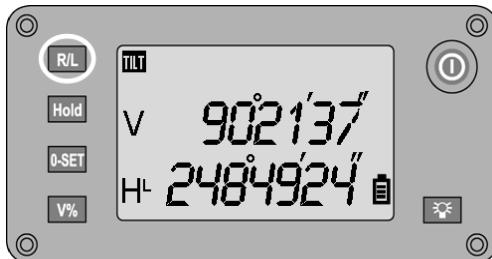
The direction of measurement for horizontal angles can be switched between right (clockwise) and left (counterclockwise) by pressing the **R/L** button.
