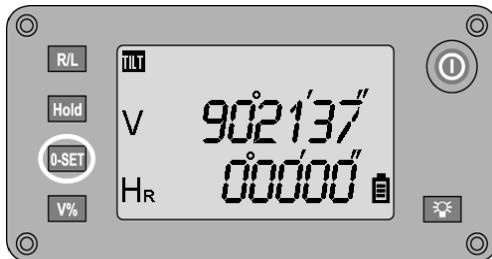
The horizontal circle can be zeroed at any time by pressing the **0- SET** button, thereby setting the reference point for the horizontal circle.
