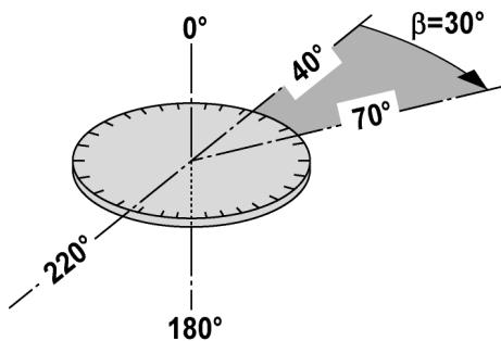
The included angle of  $70^\circ - 40^\circ = 30^\circ$  can be calculated from the horizontal circle readings of  $70^\circ$  to one target and  $40^\circ$  to the other target.
