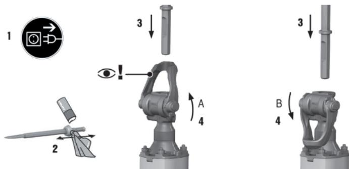
1. Apply a little grease to the connection end of the accessory tool.
