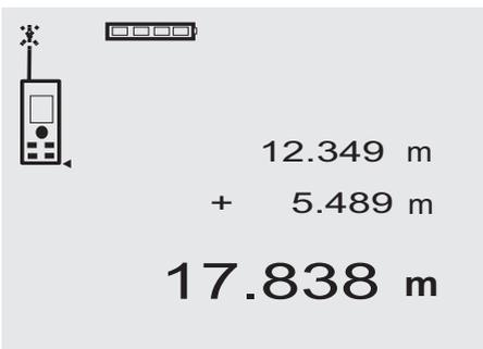
Individual distances can be conveniently added. This is useful, for example, for determining the total length of
