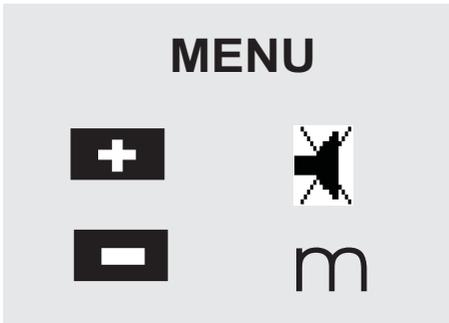
1. With the tool switched off, press the “On / off” button for approx. 2 seconds to enter menu mode.
