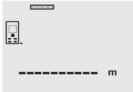
Press the “Measure” button once. The laser beam is switched on and is visible in the form of a spot on the target surface. This aiming mode is indicated in the display by a blinking laser symbol.
