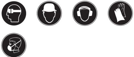
The user and any other persons in the vicinity must wear suitable eye protection, a hard hat, ear protection, protective gloves and breathing protection while the power tool is in use.
