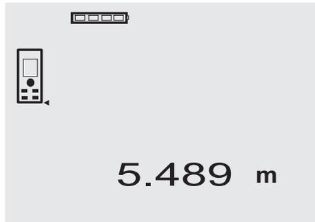
If further measurements are taken, up to three previously determined distances are shown in the intermediate result lines, i.e. a total of the last four measured distances are shown.
