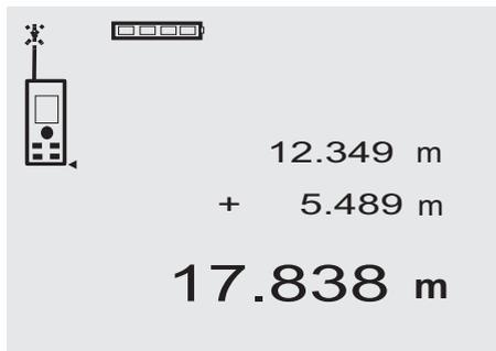
Individual distances can be conveniently added. This is useful, for example, for determining the total length of the inner face of door or window openings or for adding several individual distances that form a perimeter.
