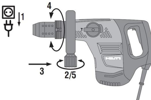
1. Slide the side handle clamping band over the chuck from the front and into the recess provided.
