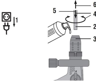
1. Apply a little grease to the connection end of the accessory tool.
