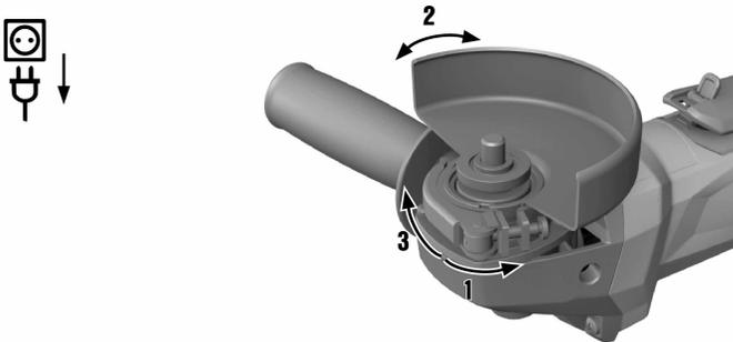
1. Release the clamping lever.
