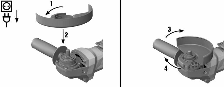
1. Open the clamping lever.
