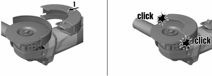
1. Position the front cover with the closed side on the standard guard and push it on until it engages.
