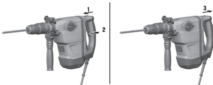
1. Push the lockbutton for continuous operation forward.
