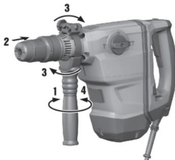
1. Release the side handle clamping band by turning the handle grip.
