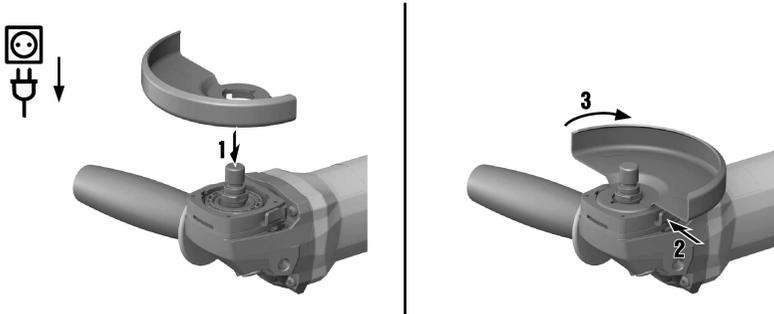
1. Fit the guard on to the arbor collar so that the two triangular marks on the guard and on the product are in alignment.
