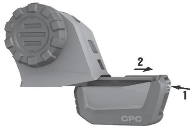
1. Press the release button at the rear of the battery.
