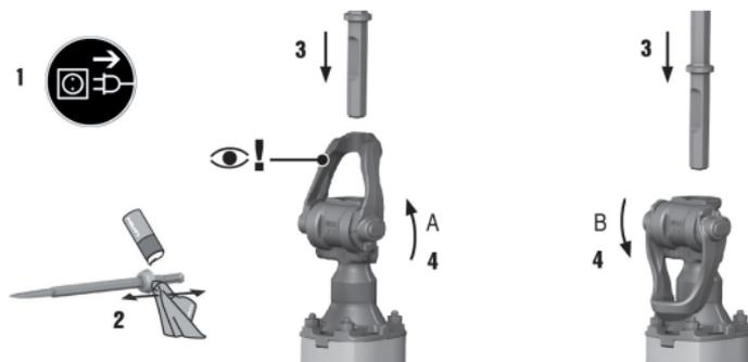
1. Apply a little grease to the connection end of the accessory tool.
