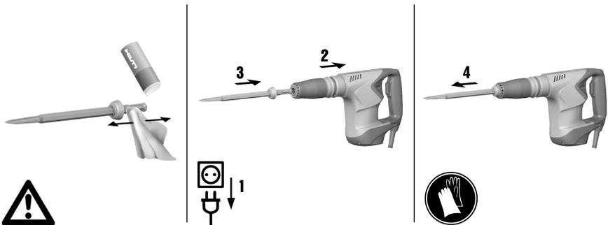
1. Apply a little grease to the connection end of the accessory tool.
