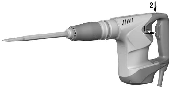
1. Press the control switch and then press the lockbutton.
