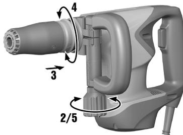
1. Release the side handle clamping band by turning the handle grip.
