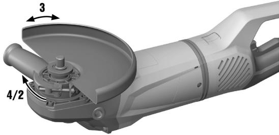
1. Release the clamping lever.
