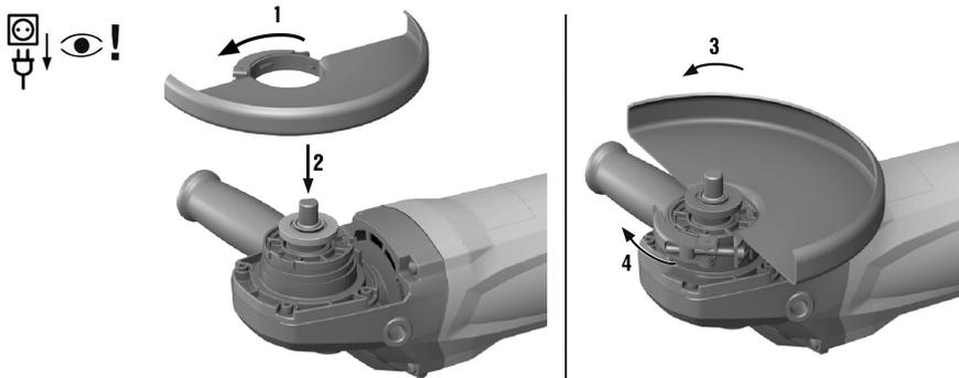
1. Release the clamping lever.
