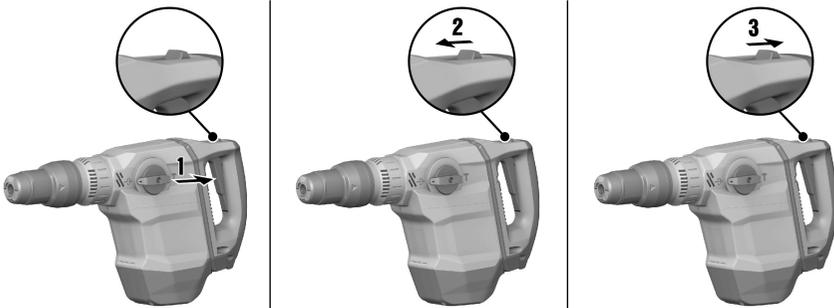
1. Push the lockbutton for continuous operation forward.
