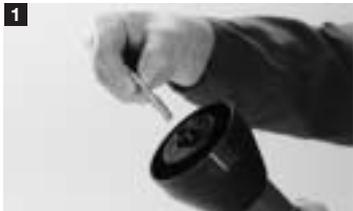
With the unloaded tool closed and locked, insert the stud or nail into the guide, head first.
