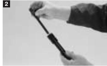
Insert the piston through the new stop ring and reassemble the tool as described.
