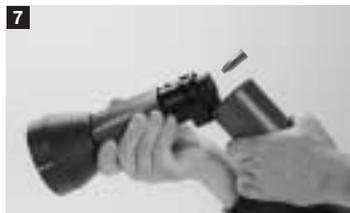
**Ejecting the cartridge case:**
