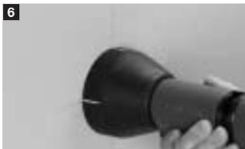
Line up the scribe marks on the protection shield with the layout lines (when necessary). Press the tool firmly against the work surface and squeeze the trigger.
