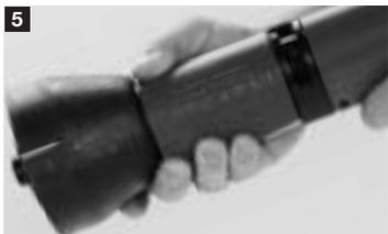
Raise the grip end to align with the front of the tool, push it forward to mate the parts, and rotate to the locked position.
