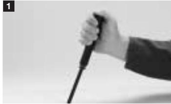
Place the extractor sleeve over the piston head, as shown, and strike the piston against a hard surface to remove the stop ring.
