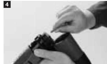
Place the cartridge into the chamber. Do not depress ejector lever.
