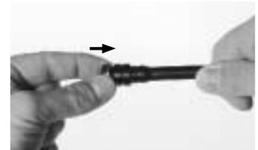
Move the piston ring by hand up to the first recessed part.
