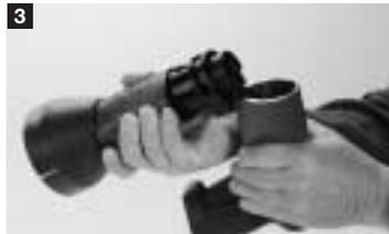
Rotate the front end of the tool to unlock it, pull it forward and lower to open the tool.
