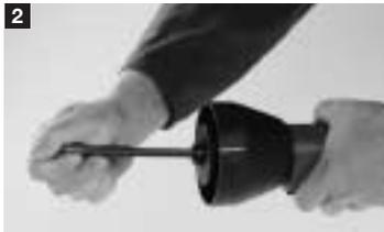
Using the ramrod, push back the stud or nail until it stops.
