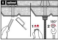
Per FM approval, the metal plate of the insert must be on the top of the deck flutes. For seismic bracing applications cut tube flush to bottom of metal deck. \*Turn threaded rod until bottomed out to ensure full thread engagement.
